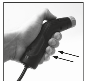
4. Actuate the lever of the trigger gun until no more water is emitted.
